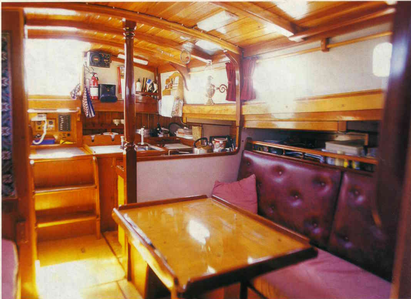
The interior is fitted out mainly in larch and mahogany, with some pitch pine coming from Ilfracombe's pier, which was built in the 1870s
